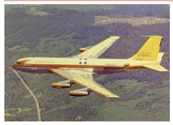
The Boeing 367-80 first flew in July 1954. It was the prototype for the 707 jet liner as well as the KC-135 tanker. Note the turbo iet engines which were rated approx. 10,000 pounds of thrust each. Later turbo fan engines were typically 17,000 pounds thrust.
